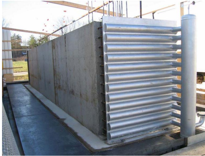
Figure 27: View of one concrete storage module, tested on the Plataforma Solar de Almeria in Spain, Image taken from [79].
